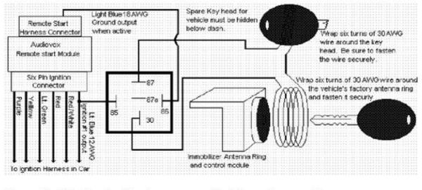
**Tips:** The light blue ignition 3 output can sink 300ma of current. Do not operate more than two standard Bosch type 332-204-150 (or equivalent) relays directly with this output, as this could damage the remote starter.
