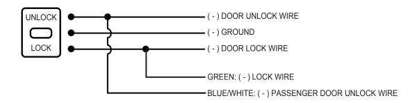
NOTE: It is necessary to go directly to the driver's door lock actuator and install a relay as shown above.
