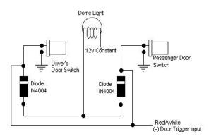
**Dome Light Supervision - Automatic Transmission Only: #5 Red/White** also provides power to the dome light circuit for **Dome Light Supervision**. **If you connect this wire to wrong polarity, the dome light fuse of the vehicle will blow.**
