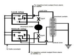
**Type 4:** Aftermarket Actuators are need for vehicles without factory power door locks requiring one door lock actuator per door. Therefore, you will need to add relays.
