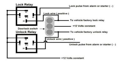
**Type 3:** Reversing Polarity doorlock systems are usually found in vehicles without a relay system. Generally, cars with two doors have these reversing polarity systems and the driver's door switch is the main switch for the system. When you encounter this type of system, you will have to add relays. Do not use the orange and blue wires directly since these are 200mA output only.
