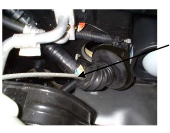
Lubricate the pilot feeder and alarm harness with liquid hand soap.
