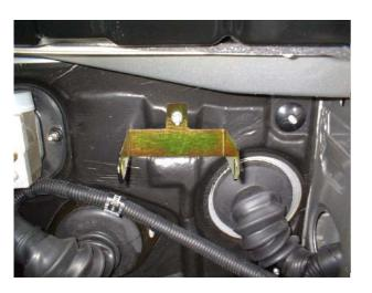
Locate the M6 stud located on the bulkhead and secure the siren bracket using the M6 flange headed nut provided.
