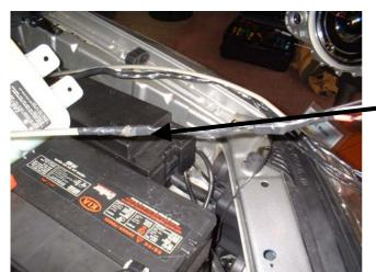
Feeding the alarm harness into the car via the main grommet will require great care as space is restricted.
