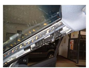
Remove the R/H (O/S) A post trim and position the ultrasonic head as shown.
