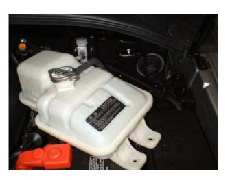
Remove the three M6 nuts securing the cooling system header tank. Lift the tank and position to one side as shown allowing access to the N/S bulk head area.
