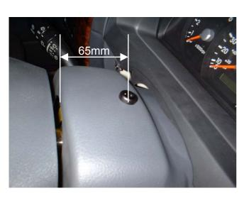
Remove the steering column upper housing and drill a 10mm hole 65mm from the front edge and in a central position.
