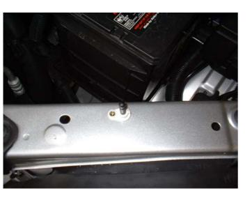
Fix the bonnet switch in position using The M3x10mm long C/S self tapping screw provided.
