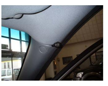
Replace the R/H A post trim and position the ultrasonic head as shown.
