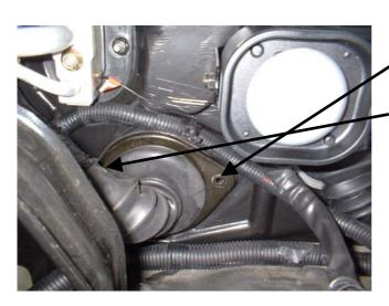
Remove the two M6 nuts securing the main grommet retaining shroud.
