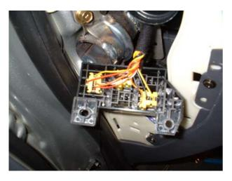
Remove the relay panel and turn upside down to expose the wiring as shown.
