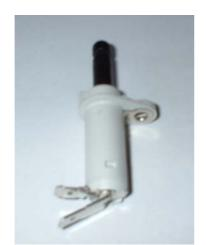
The bonnet switch wire must be connected to the lower of the two terminals.
