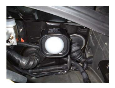
Secure the siren in position onto the bracket using the two M6 sq headed bolts and M6 nyloc nuts.
