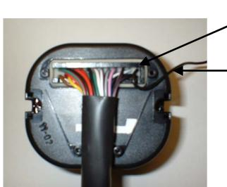
Fit the multi pin harness connecter into the siren block and ensure it is fully home.
