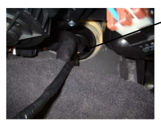
Pull the alarm harness through into the car leaving a little slack from the siren to the entry point at the trunking.
