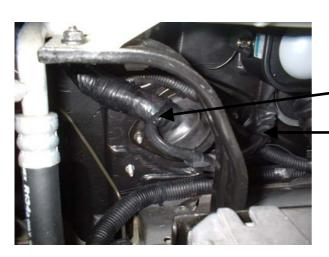
At this point, re-tape the grommet trunking to the main harness ensuring that the alarm harness is also taped securely at the entry point.
