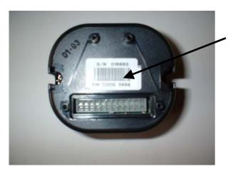
Secondly, stick the top part of the identification label over the bottom part as shown.
