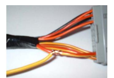
Wind the end of the alarm harness wire around the un-insulated part of the vehicle wire 2 to 3 times until it is firmly fixed.
