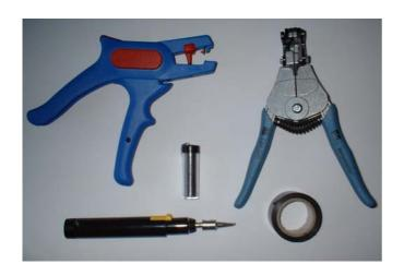
Tools to use are shown opposite and include: wire cutter & end stripper, wire stripper, soldering gun, self fluxing solder And amalgam tape.
