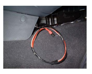
Feed the LED wire and the R/H (O/S) ultrasonic wire behind the passenger glove box and under the centre console into the driver's footwell area as shown.
