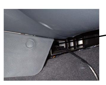
Connect the R/H (O/S) ultrasonic wire and th LED/PIN code wire into the alarm harness.
