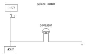
H1/8 BLACK (-) chassis ground connection: Connect this wire to bare metal, preferably with a factory bolt rather than your own screw. Screws tend to either strip or loosen with time. All components, should be grounded to the same point in the vehicle if possible.
