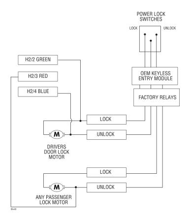
**NOTE:** It is often easy to access the passenger unlock wire going to the rear door motor on the driver's side.
