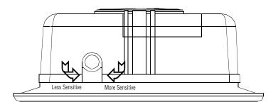
There is a dual-stage shock sensor inside the control module. Adjustments are made via the rotary control as indicated above. Since the shock sensor does not work well when mounted firmly to metal, we recommend against screwing down the control module. The full trigger of the onboard shock sensor reports zone 2. See Table of Zones.
