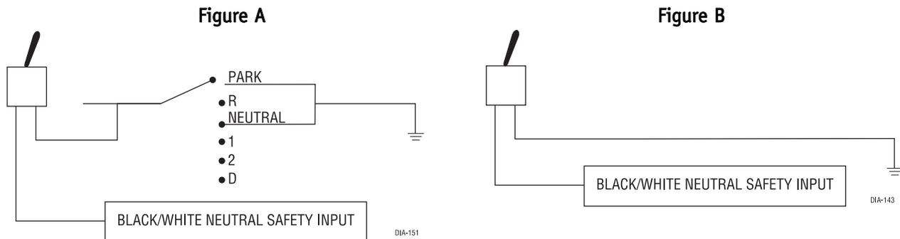
**IMPORTANT!** Always perform the Vehicle Safety Check section of this guide to verify that the vehicle cannot be started in ANY drive gear and that the override switch is functioning properly.
