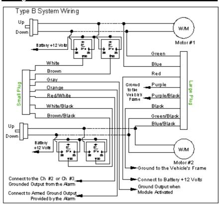
Note: The wire positions shown the diagram above do not match the actual wire positions on the plugs.
