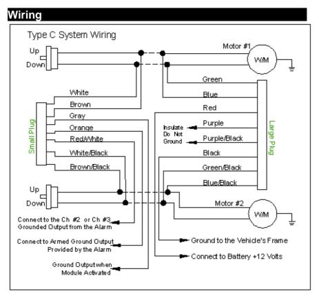
Note: The wire positions shown the diagram above do not match the actual wire positions on the plugs.
