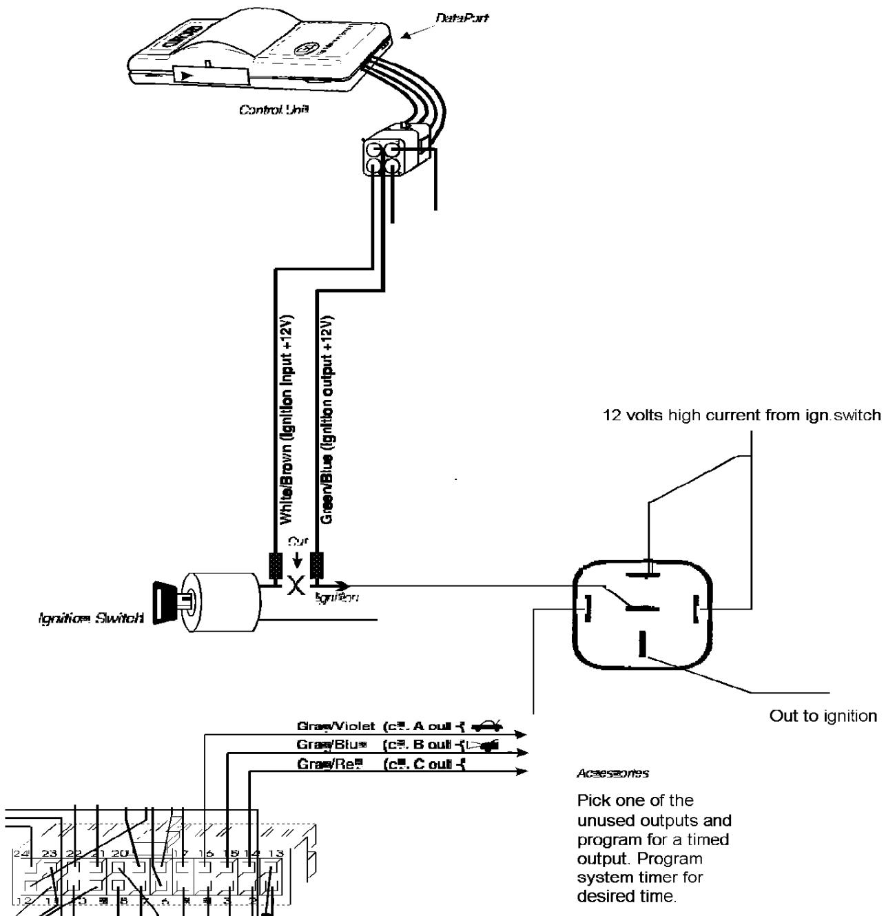
While key is still on transmit appropriate channel and then turn key off vehicle will continue to run for the time you set. On some vehicle you may need to power more than one ignition.
