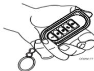
**4. Transmit.** While holding the Valet/Program switch, press the
