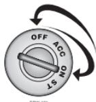
2. **Ignition.** Turn the ignition on, then off. (The heavy gauge PINK wire must be connected.)
