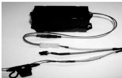
4. Plug the back-up battery into the main wiring harness.
