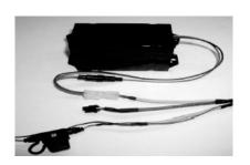
4. Plug the back-up battery into the main wiring harness.
